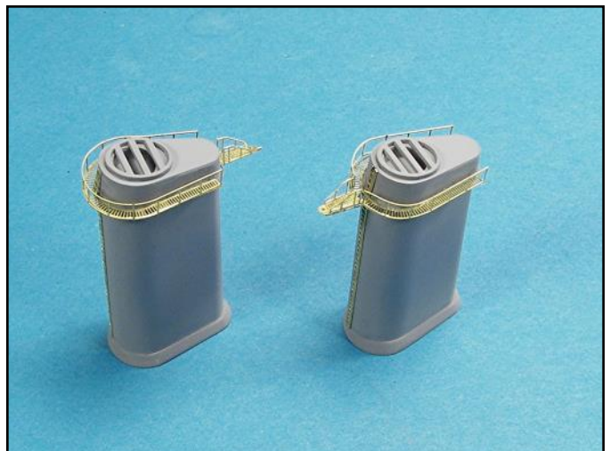
The smoke stack platforms were then glued to their respective stacks. Be careful, as the photoetch assemblies are different for each smoke stack.
