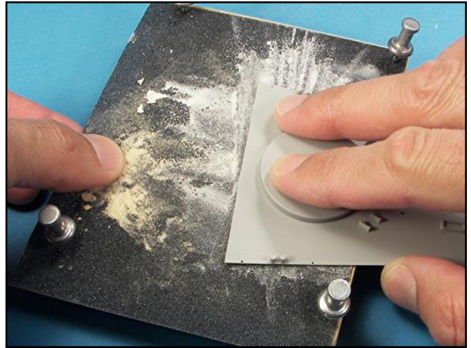
The remaining positioning tabs on the undersides of the decks were sanded off. A new lip will be added on each deck section.
