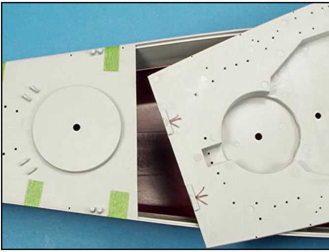
This kit's main deck is in three sections so the first step is a test fit between the sections and the upper hull. The positioning tab extensions on the undersides of the decks have to be removed for a tighter fit along the deck seam lines.
