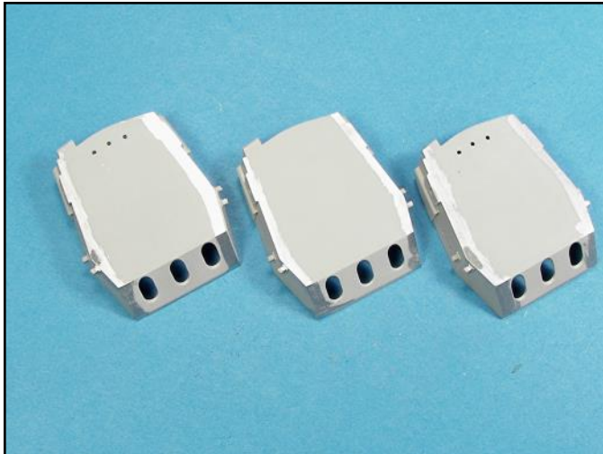
The seam lines were checked with silver paint and additional super glue applied in needed areas. The sanding and finishing process was then repeated until the seams disappeared.
