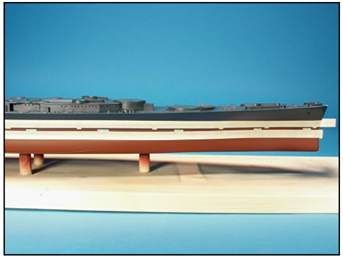
Masking tape sections were used to set the locations height and the thickness of the black boot strip.
