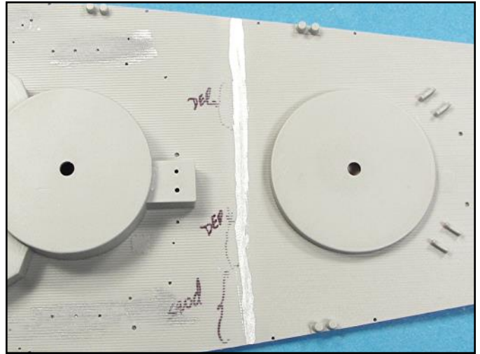
The forward seam line was wet sanded first then the depressed surface areas were wet sanded. Silver paint was applied to check the seam and no additional super glue was required.
