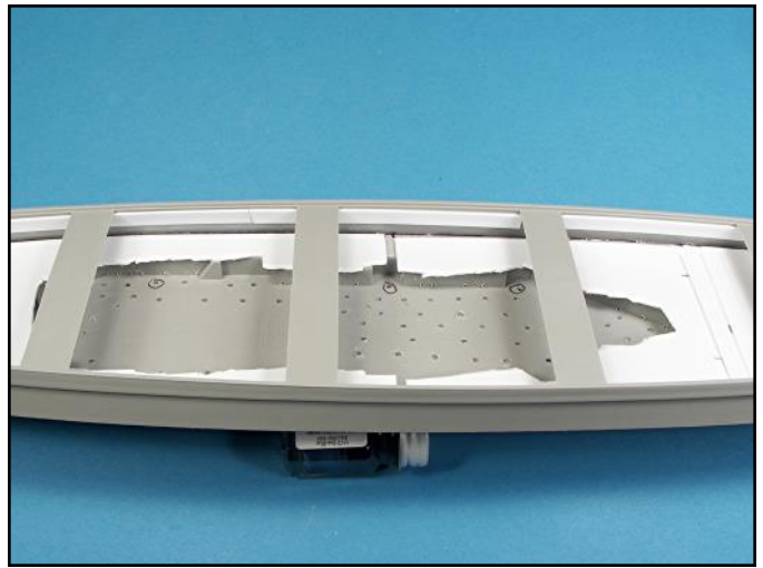
To stop the upper hull from flexing, laminate .030 x .250 inch strips to the inside surfaces.
