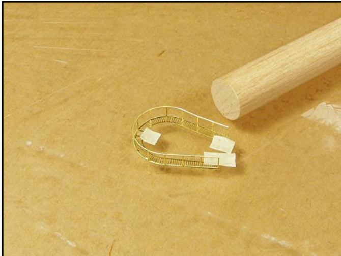
To work with the delicate smoke stack platforms, carefully tape them to a piece of Plexiglas, shape the railings and glue them into place.
