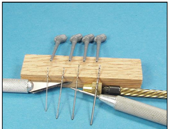
The barrel tips were hollowed out using various sizes of drill bits. Use a pin vice to center punch an indentation in the tip of each barrel and then use the smallest drill bit for the first hole and then graduate to progressively larger bits.
