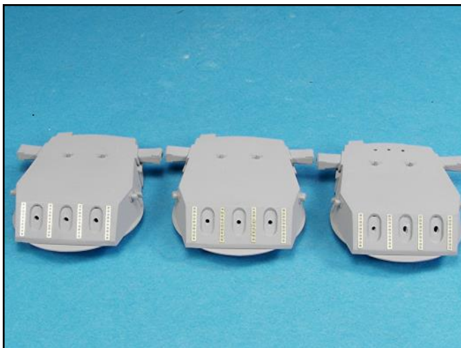
The locations of the turret vents were marked, holes drilled and then .035 inch round stock was cut and glued into place. The optical range finders were added, the turrets primed and then the photoetch ladders were added.
