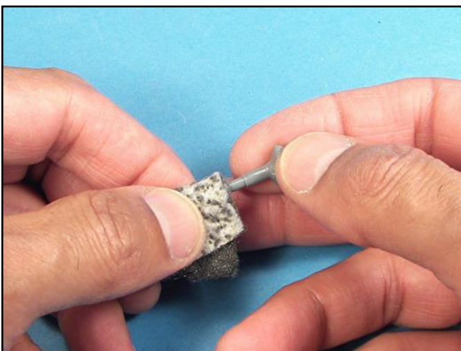
To polish the surface of the barrels and restore the round shape, 0000 steel wool pads were wrapped around the barrels and the plastic was rotated inside the pads.
