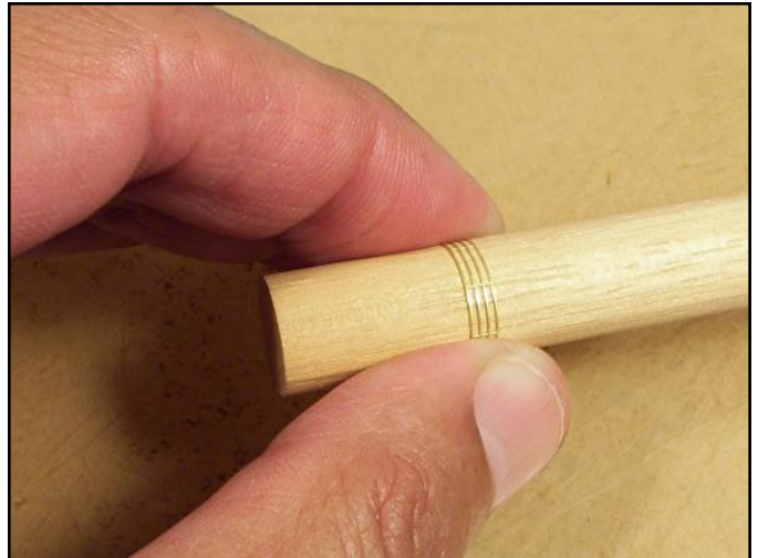
To achieve curves use wood dowels and the stems of drill bits. Use a diameter slightly smaller than the one you need, as the curve you form in the railings will spring back some resulting in a slightly bigger radius.
