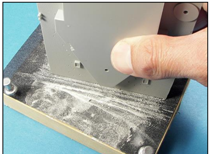
The excess plastic on the aft center deck section was slowly sanded down by adding more pressure to the side that had the most plastic to remove. The deck was form fitted into place by sanding, test fitting and sanding again.
