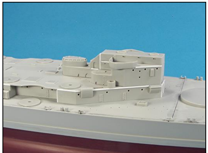
The aft superstructure was attached to the 01 level to make it easier to paint. Note the .030 inch half round sections applied to the superstructure assembly to hide seams that would be difficult to fix.
