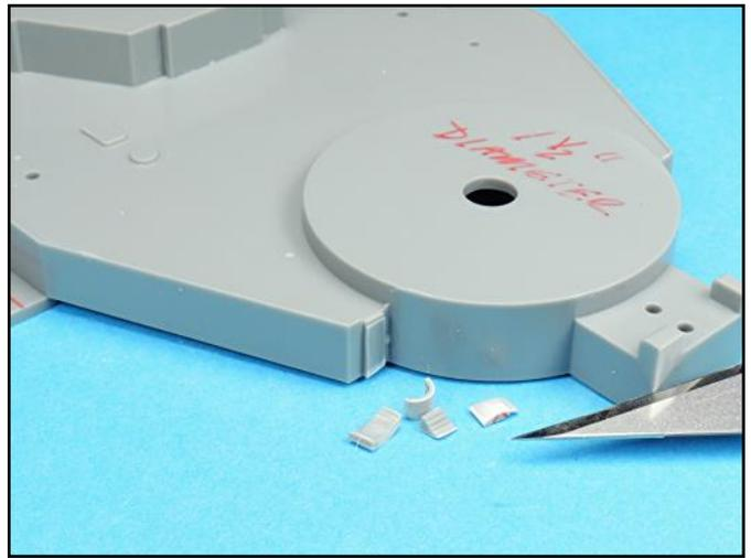
The molded on inclined ladders were shaved down with a sharp number 11 X-Acto blade.
