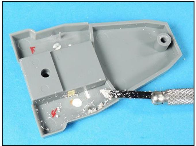
The plastic was lightly scraped with an X-Acto stencil knife. Due to the blade angle some deep scrape marks were made into the plastic.
