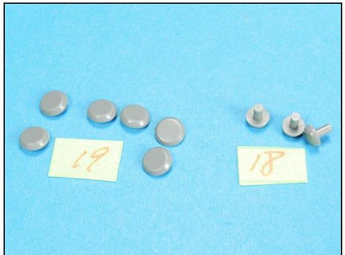
Be careful when removing the tree attachment stubs from these round vent covers so that the shapes will not be distorted.
