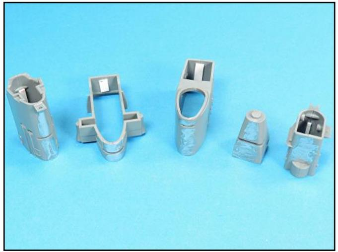
All of the superstructure assembly seams were checked with silver paint for any remaining flaws.
