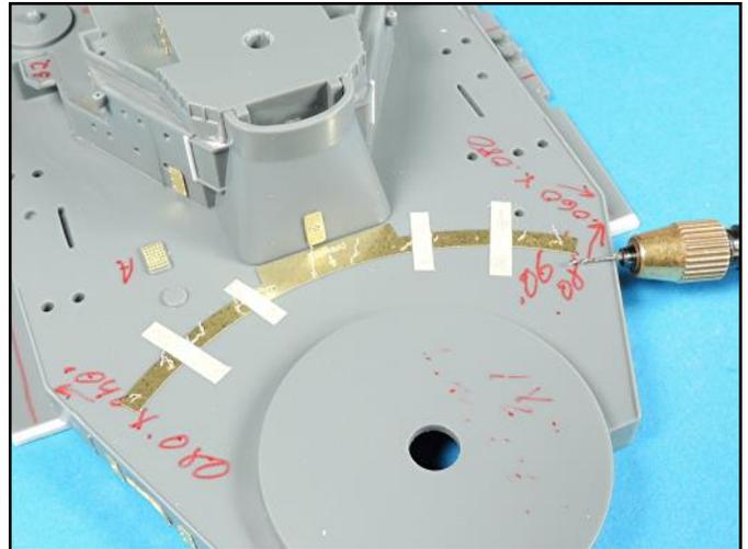
The Gold Medal Models deck railing gauge behind the number 2 turret was carefully set in place with tiny strips of masking tape and the holes drilled out with a .0145 inch (#79) bit.
