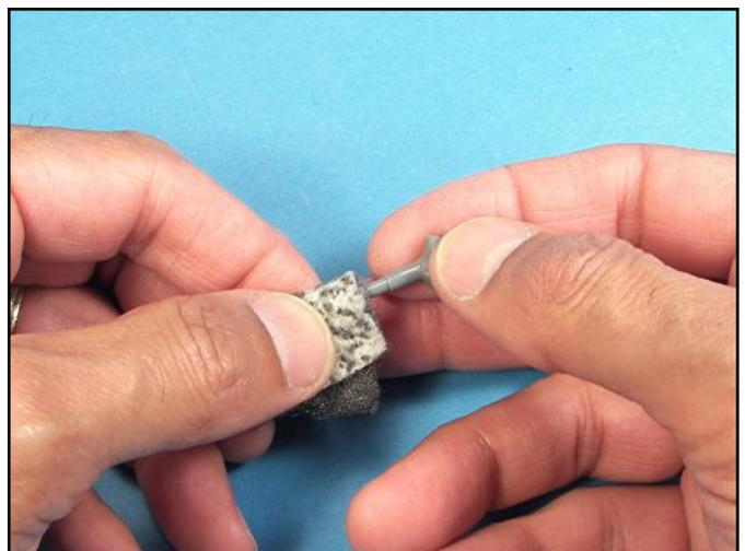
The round shape of the guns can be restored by rotating the barrels inside 000 steel wool pads. This also polishes the plastic.
