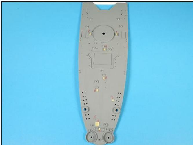
The Gold Medal Models deck hatch details were carefully glued into place using tiny drops of slow set super glue. Each part was picked up with a toothpick with a flat end that was moistened and carefully positioned.
