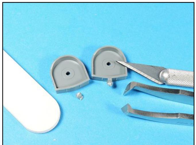
The tree stubs on the 16 inch turret 40mm Bofor platforms are attached to the upper edges of these parts where there is a lip. Use snippers to remove the stubs and then carefully smooth the edges with a sanding stick.
