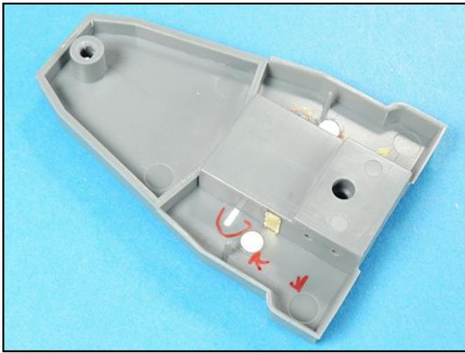
This part has a round mold punch out and a depression for an inclined ladder part. Both were filled with a tiny piece of plastic and a disk punched from a Waldron Punch tool and super glued into place.
