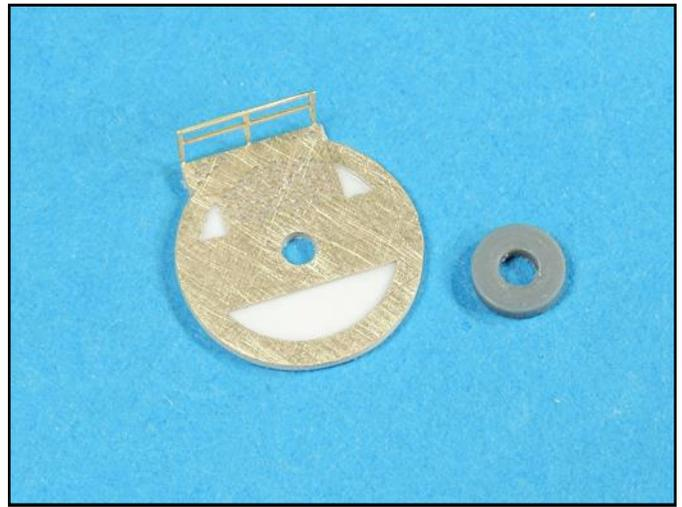
With a hole drilled through the new base with a .052 inch bit (#55), both parts can easily be lined up.
