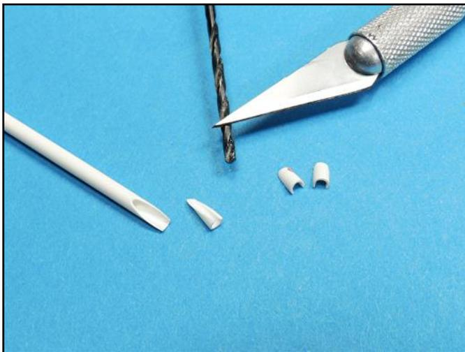
Anchor chain deck hole covers were made using 1/8 inch tubing. The inside diameter was made larger with a .067 inch bit and then then cut at an angle. It took several tries to get two of the same angle and length.
