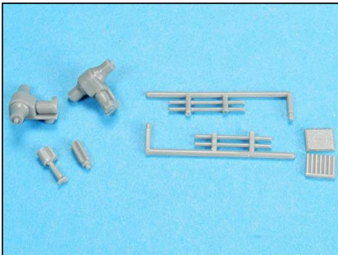
Be sure to check each part for a mold line and carefully scrape them off with a sharp number 11 X-Acto blade.
