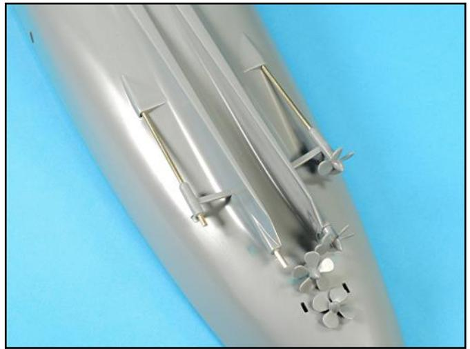
Each propeller was marked on the inside of a blade so they would not get mixed up. The shaft openings on the propellers were carefully opened up to accept the new shaft diameter.
