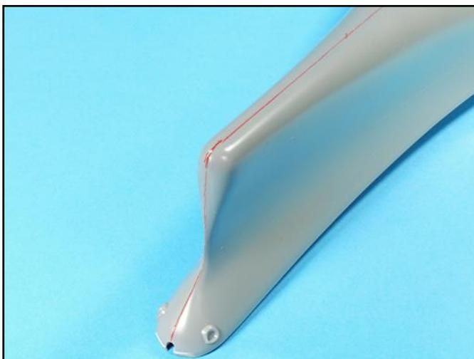
The mold line on the bow will need to be carefully scraped with a sharp number 11 X-Acto blade and then wet sanded smooth with fine grit sandpaper
