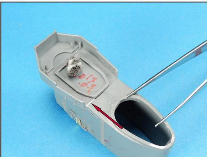
The voids between these two parts were filled with tiny lengths of plastic strip super glued into place and lightly scraped and then polished with a 0000 steel wool ball.
