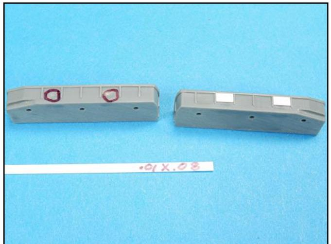
There were some indentations in the surface of the parts on these two deck inserts. The indentations were hidden with lengths of .01 x .08 plastic strip.
