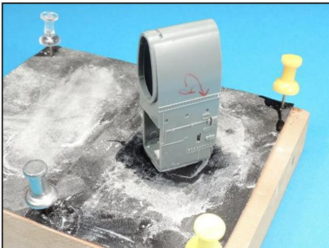
The seam and the depressions were wet sanded smooth by running the assembly across a stationary piece of sandpaper.
