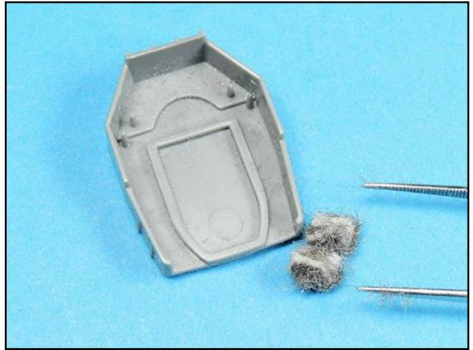
The deck surface was polished with a 0000 steel wool ball held with a pair of tweezers.
