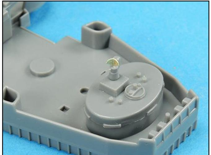
This tiny Mk-27 radar was shaped with a micro file handle.
