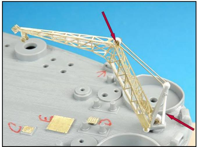
The photoetch pulley assembly and the cable frame have been super glued into place. A strong back for the "A" frame was made from .030 inch diameter rod and the tiny photoetch bracing (top arrow) came from the Eduard set.
