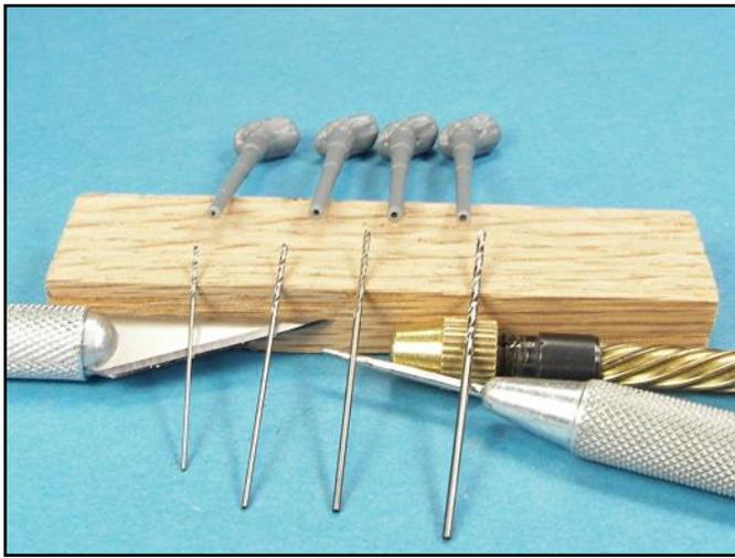
Center punch the tip of each barrel and drill out the tips. Start with a .028 (#70) inch bit and work up to a .039 (#61) inch bit. If you try to remove too much plastic too fast you will collapse the sides of the plastic ruining the part.
