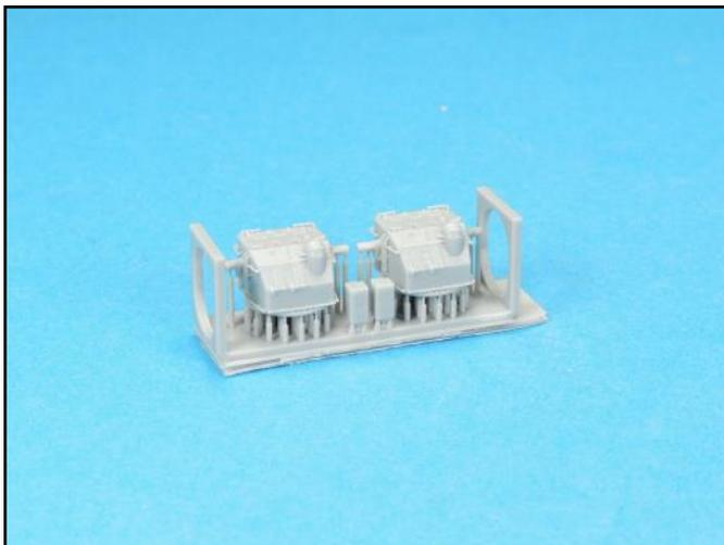
This is how the Black Cat Models 3D printed Mk-37 radar bases are set inside the print frame. The rectangular shapes glue into the backsides of the bases.
