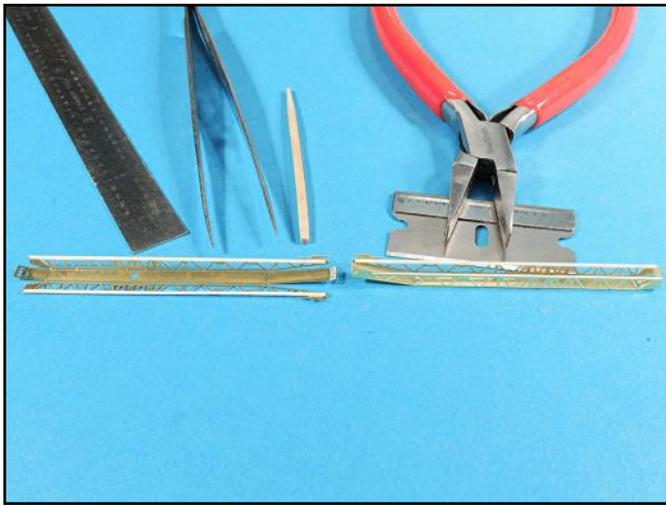
The side frames were bent up using a metal ruler and a single edge razor blade. The front and rear plates were bent up using tweezers.
