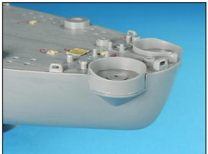
The seams on the aft 40mm bofor tubs were filled with several applications of super glue.
