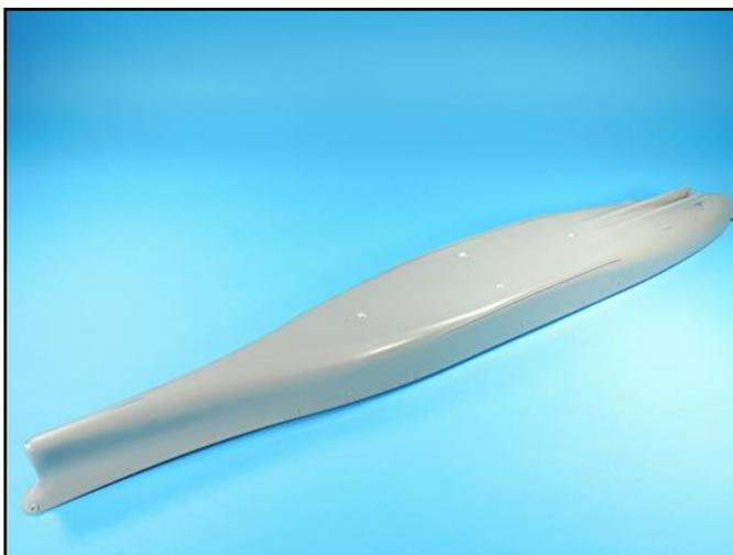
With the hull cleaned up, the pedestal holes drilled out and the anchor holes and shaft locations completed, its time to start working on the main deck.
