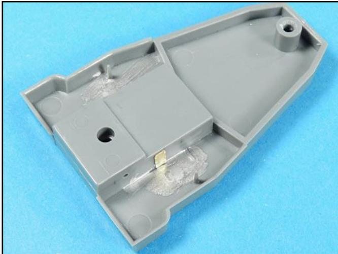
After wet sanding and polishing, the silver paint detected additional scrape marks that could not be reached for adequate sanding.
