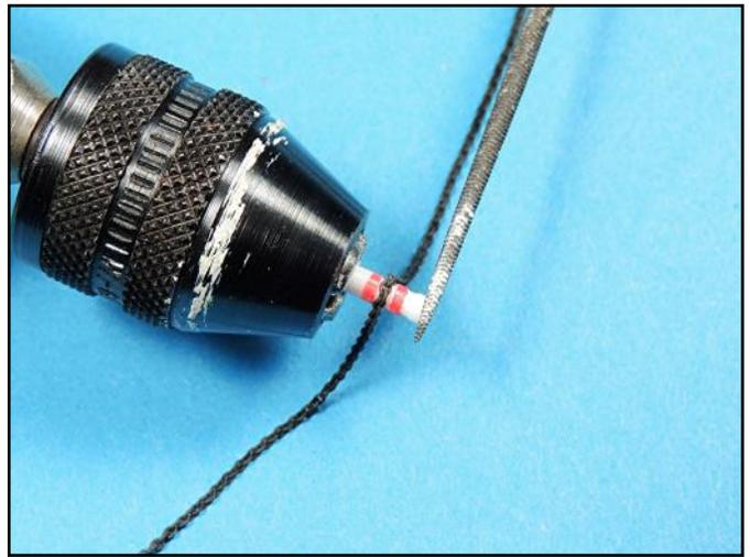
The depth of the cut into the plastic rod was checked with the HO scale chain. With the top and bottom of the capstan marked, the cuts were done with a Northwest Short line chopper.
