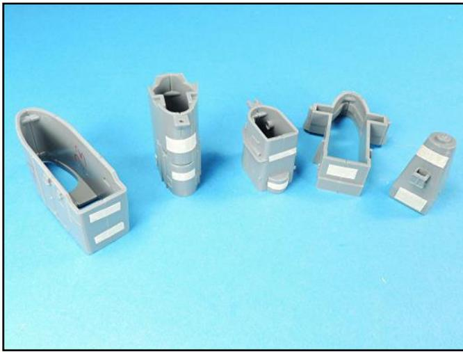
The upper superstructure gluing surfaces were all flattened so that the seams would be tight. Each assembly got several strips of masking tape to hold the halves tightly together.
