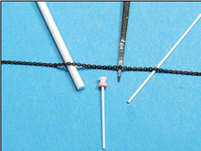
The mine sweep chain capstan is complete. A .026 inch hole was drilled into the bottom and a length of .025 inch diameter plastic rod inserted. This rod will serve as a locating pin.
