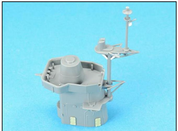
The upper mast was attached with Testors red tube glue, the part was positioned and then super glued into place. A cut disk (.010 inch thick) was made using a Waldron Punch Tool for additional yardarm rigging.
