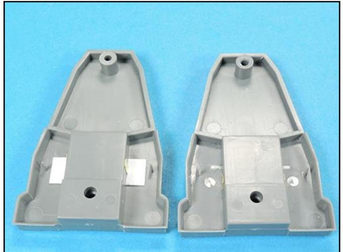
The better solution was to glue a length of .010 inch thick plastic to cover these indentations.
