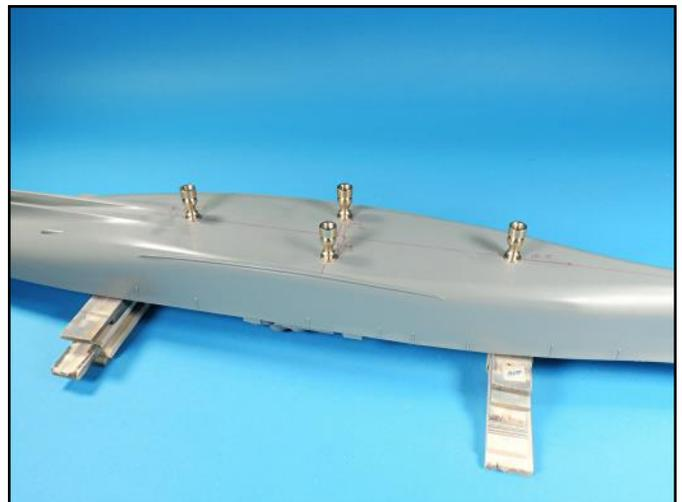
The brass pedestals were super glued into place and allowed to set and dry for several hours. Note the stacks of balsa wood strips held together with masking tape to elevate the assembly
