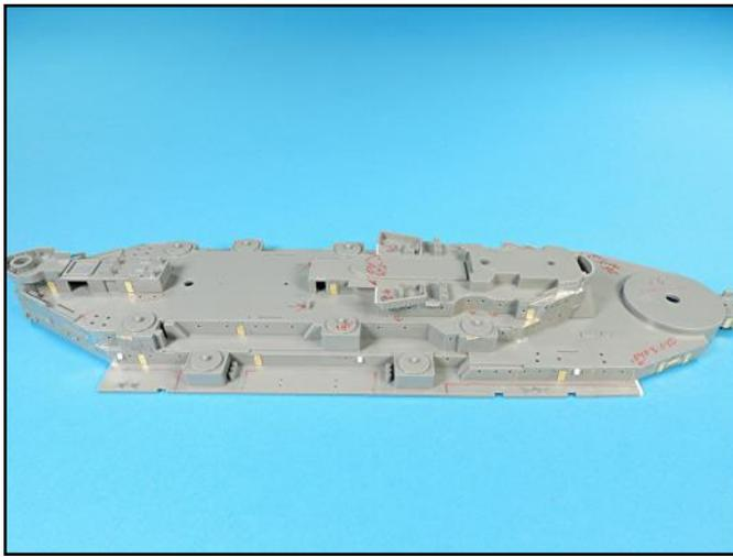
The forward and aft upper deck sections have been glued into place.
