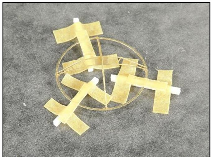
To simplify construction, raise the ring so that the frame steps will sit correctly on the ring. Tiny drops of super glue were applied with a .012 diameter stiff wire applicator.
