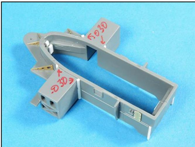
To hide the voids between the main assembly and the added framing detail, small lengths of .030 inch quarter round strips were glued into place.
