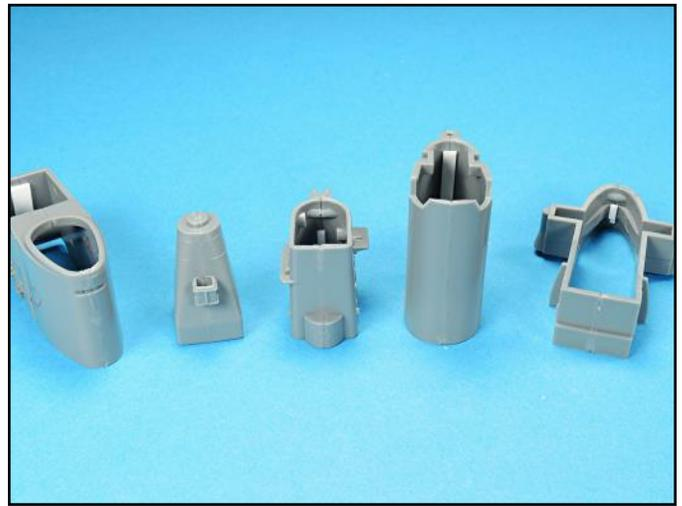
Tiny beads of super glue were applied along the seam lines with a .012 inch diameter stiff wire between the masking tape strips. After the glue dried the tape was removed and additional glue was applied.
