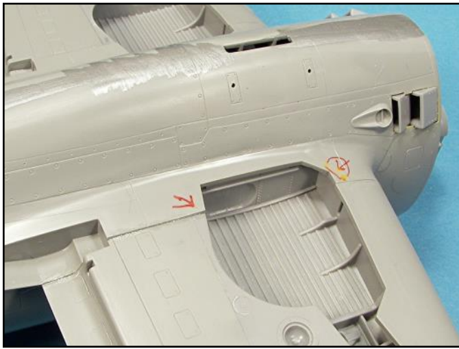
The port side wing underside had an even higher step that needed to be sanded.
