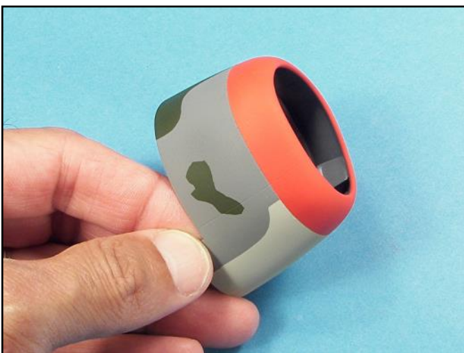
The next step was to cut out some random shapes for the dark green color. The demarcation lines between the different colors are very sharp thanks to careful masking.
