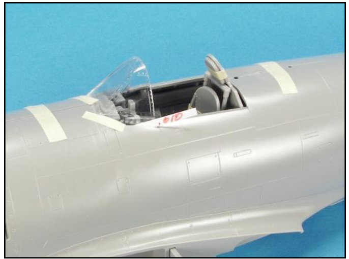
I also checked the fit of the canopy windscreen and found that the port side had a gap which would need to be filled with .010 inch strip.
