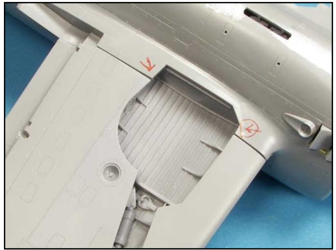
There was also a gap on the undersides, sink marks and a height difference between the wing and the fuselage.
