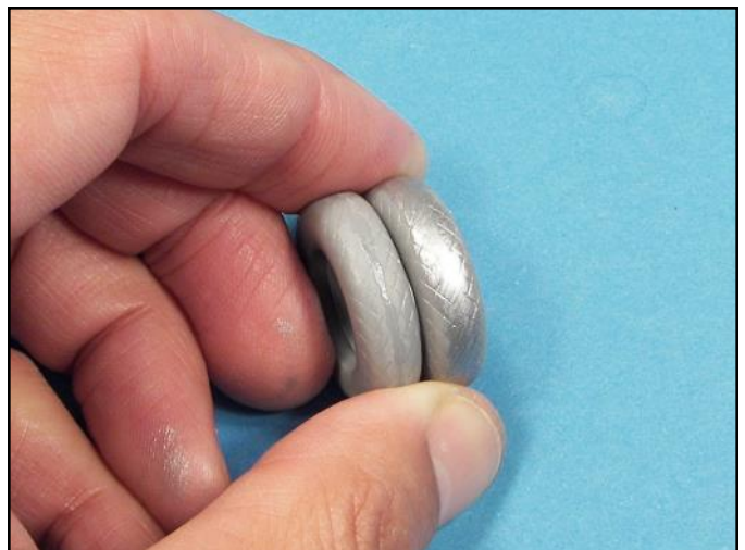
The bead of super glue is almost invisible on the left tire and the right tire has been checked with silver paint.
