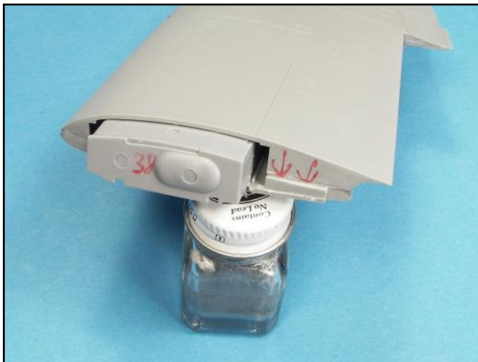
The culprit was a tab on the inside area of the wing attachment surface which needed to be cut down and reduced in size.
