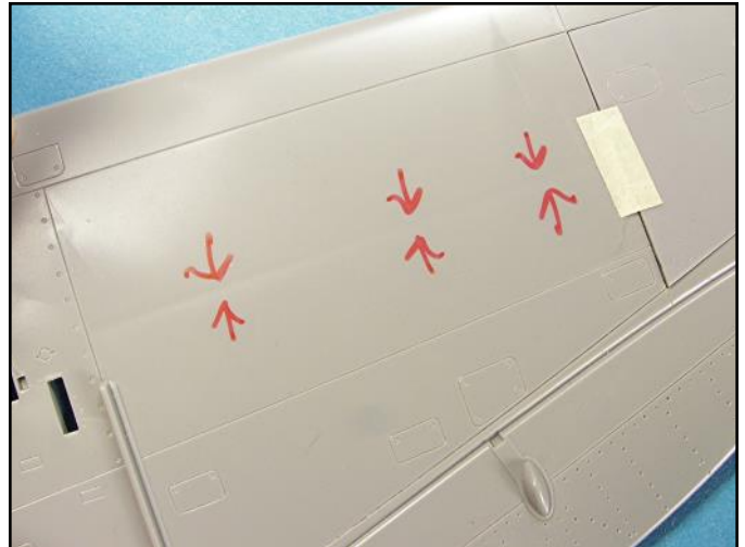
There are stringers on the inside of the wings to add strength however there are also depressions on the wings surfaces which will need to be sanded out.
