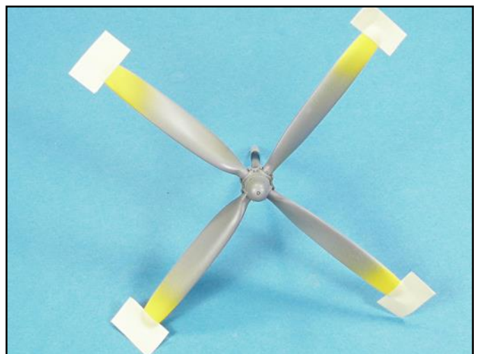
The tips were then masked off. Be sure that the masking tape positions on both sides of each propeller blade match. Also, be sure the masking tape is pressed flat onto the surface so there is no paint bleeding under the tape.
