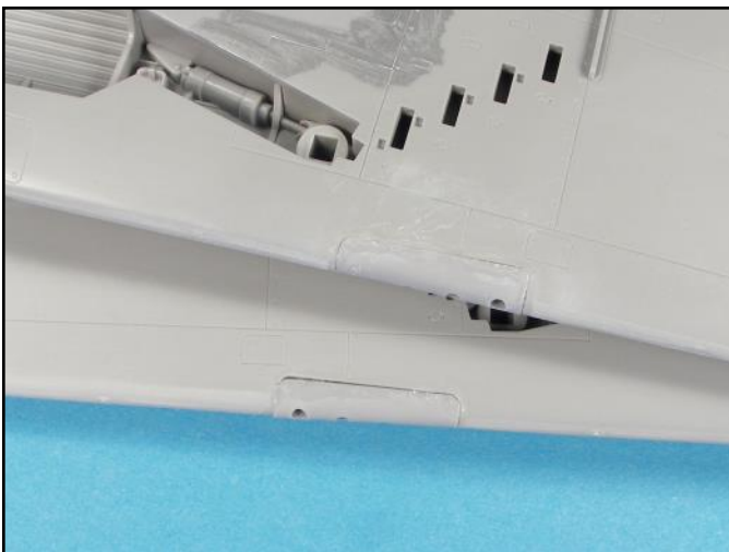
The covers for the wing guns did not fit well on the leading edges of the wings. It took several iterations of scraping, sanding and applications of super glue to get them contoured correctly.
