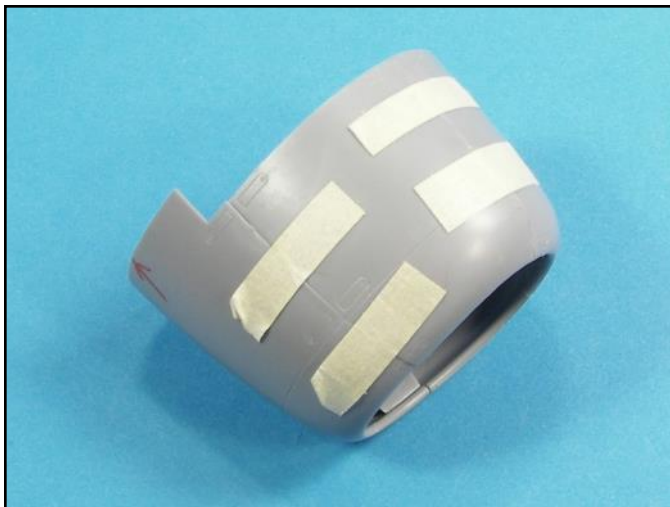
It took several attempts to get the engine cowling panels to line up correctly and taped together. I did not glue the lower panel in place, because it is the solution to the step problem between the cowling and fuselage.
