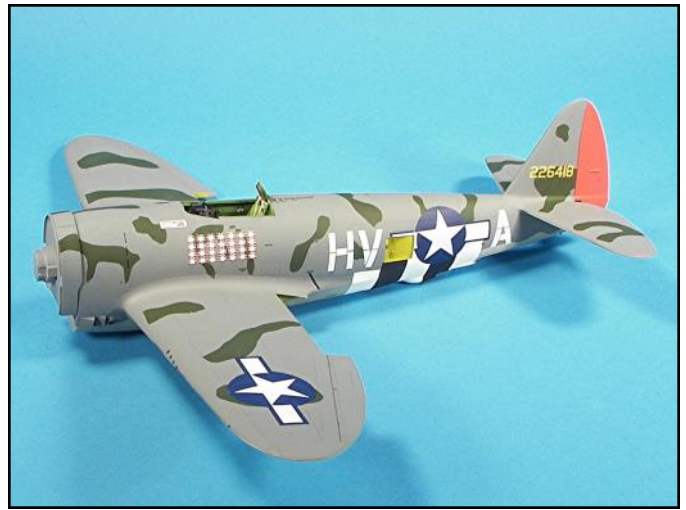
The entire model was then given two coats of Testors clear dullcoat.
