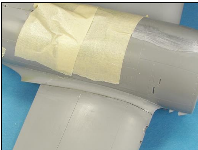
The upper wing seams were very tight and only needed a few applications of super glue and wet sanding to get them smooth.
