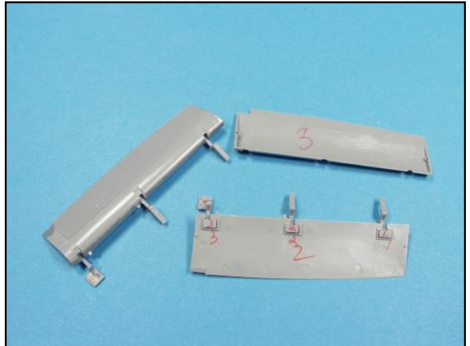
I marked the hinges so they would not get mixed up. I glued them into place and then closed each hinge, taped them together and ran a bead of super glue along the seam line. Light scraping and sanding fixed the seams.
