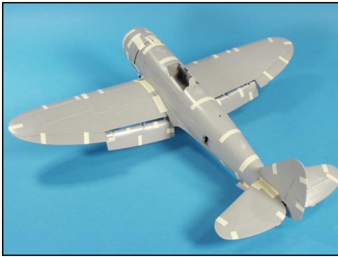
All the major components were cleaned up and taped together to check the fit and identify areas that would need attention.
