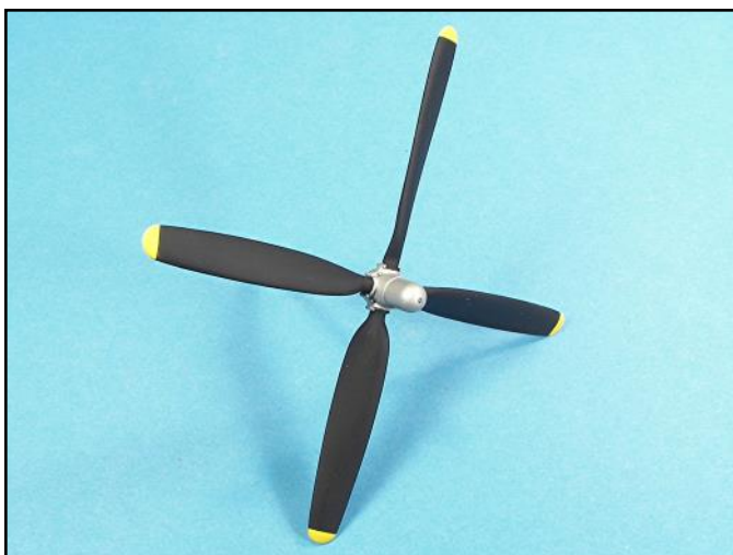
With all the masking tape removed, the propeller has very sharp demarcation lines between the colors.
