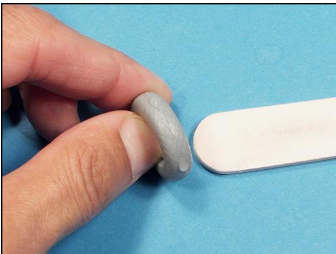
I used a sanding stick to smooth the super glue along the seam lines on the tires. I also kept the surface wet so that the tread detail would be minimally impacted by the sanding.
