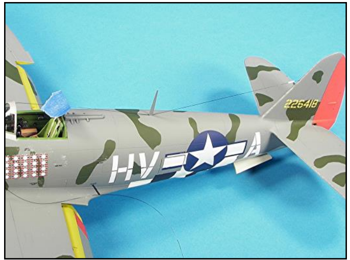
I also drilled a tiny hole through the vertical antenna and used nylon thread colored with an indelible marker to depict the antenna wire. The white insulator located near the tail was made from a short length of plastic rod drilled out.
