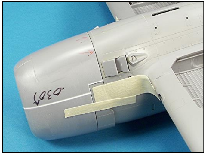
A final test fit showed that the step between the cowling and the fuselage has disappeared. I had to do a little sanding along the edges of the cowling to get a tight fit.
