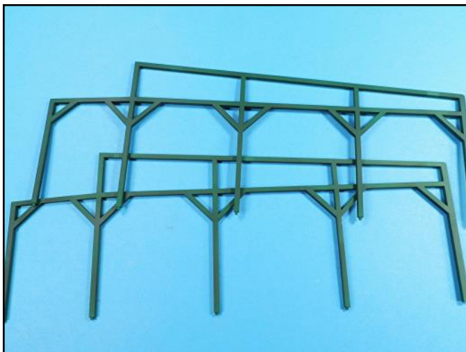
All sides of each frame received dustings of black pencil dust and then the parts were given a coat of Testors clear dullcoat.
