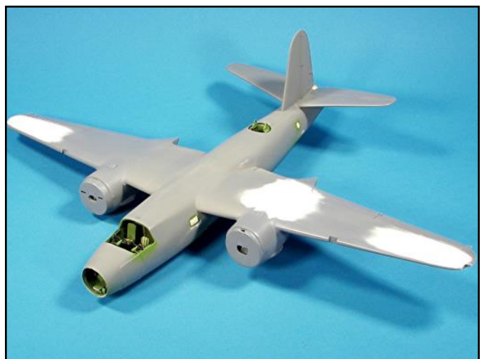
The completed assembly is now ready for masking and a final coat of primer.
