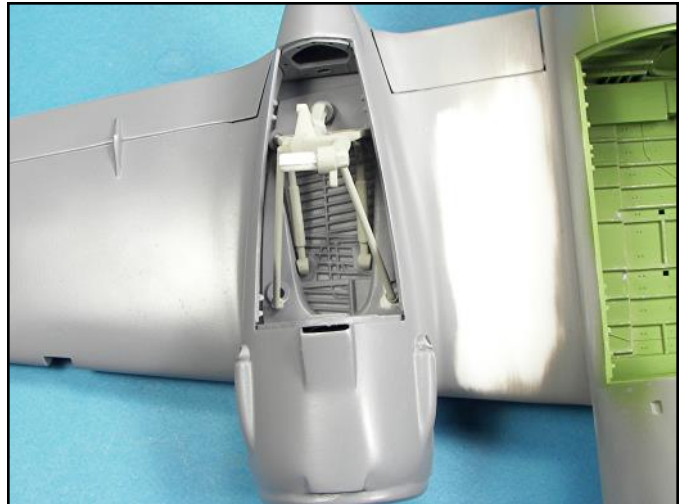
I didn't like the way the starboard splice job looked so I decided to glue the legs in place and cover the locator holes with small disks punched out with my handy Waldron punch tool.
