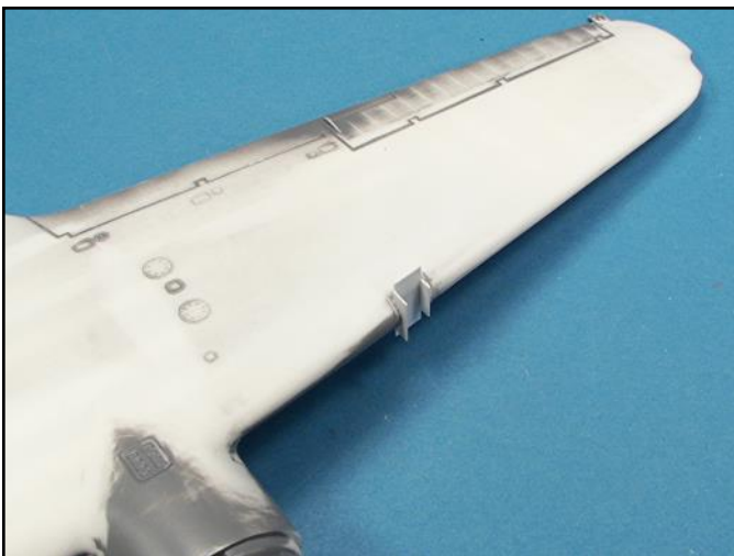
The wing lights on both wings were just holes so I boxed them in with plastic strip.
