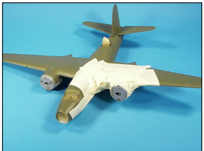
To paint the engine exhausts, I started to mask off the areas around them so that there would be no chance of the paint ruining the surface colors.
