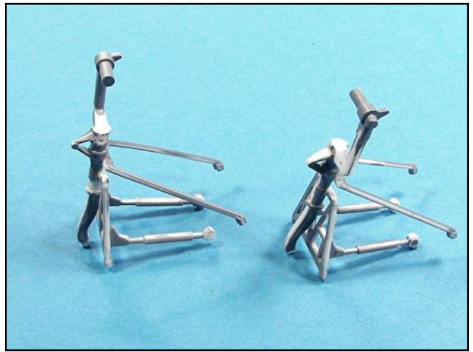
I positioned the landing gear inside the engine nacelles, taped the parts together and then added tiny drops of super glue to secure everything together. I also noticed that the forward legs were too long for the locator pins inside the nacelles.
