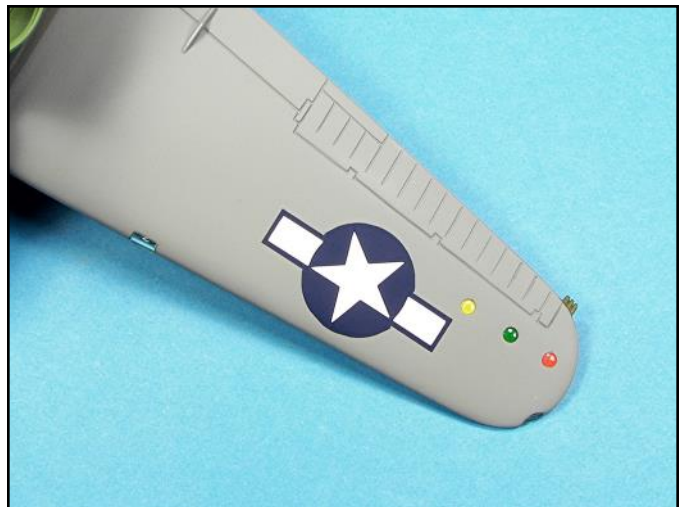
The formation lights were painted on the backside of the clear parts and then attached with white glue.
