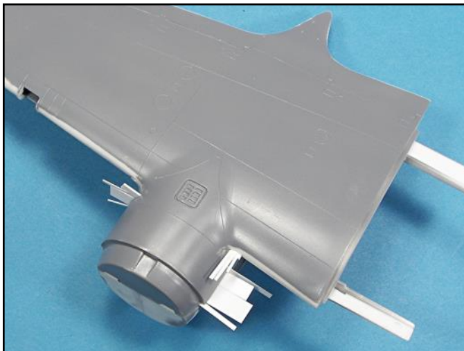
The starboard wing had a lot of voids to fill in between the engine nacelle and the wing. Various sizes of plastic strip were used. I positioned all the strips in place and then applied super glue to both sides of the strips.
