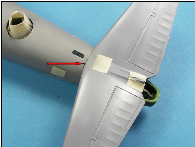
There was also a void at the front area of the attachment point of the elevator and the fuselage.
