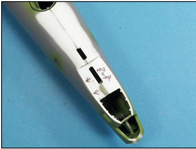
The elevator assembly sat at an angle so I added some shims to the gluing surface to level it.
