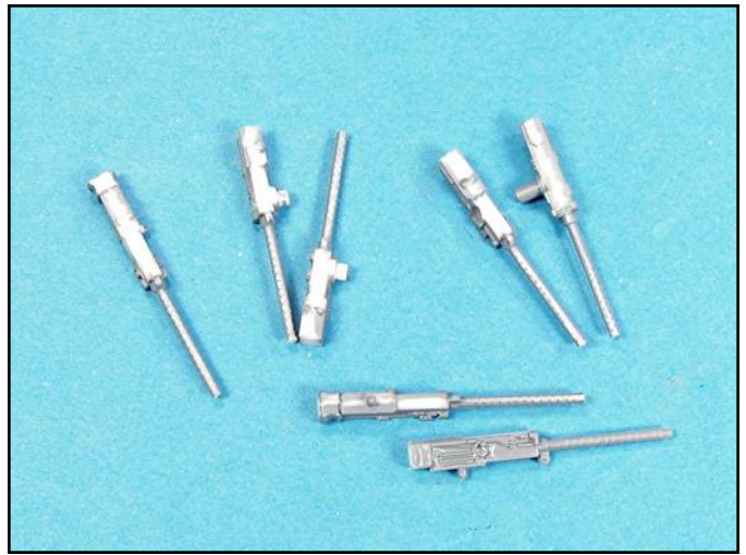
I cleaned up the 50 caliber guns and carefully scrapped off the mold lines.
