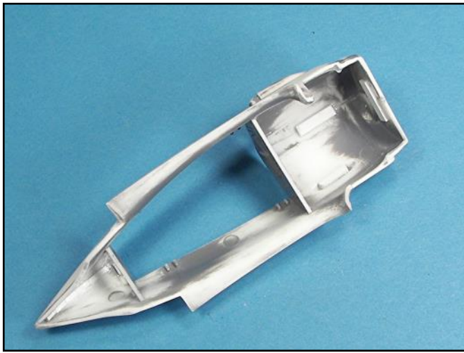
The engine nacelle sub-assemblies are now complete with the addition of the interior bulkheads.
