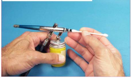
To ensure that all of the paint is gone from the tiny airbrush tip I run a thin stiff brass wire through it. This usually removes the tiny paint particles that tend to cling to the inside area of the tiny tip. I also keep this length of wire handy during airbrush sessions to clear clogs in the tip.
