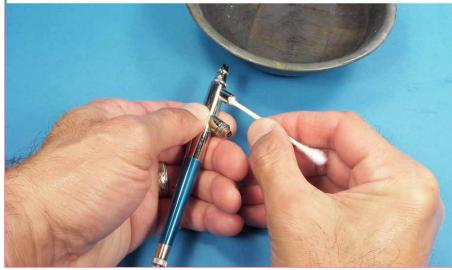
Sometimes during airbrushing the tip can collect paint which will splatter all over your model. This usually happens when the paint is slightly thicker than it needs to be or when you are airbrushing large models that take some time to complete. I frequently check the tip and wipe it with a Q-Tip to remove these dangerous globs of paint before they create a disaster.
