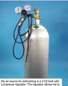
My air source for airbrushing is a CO2 tank with a pressure regulator. The regulator allows me to adjust the air pressure between 1 and 100. The air is always dry and its very quiet. This tank can last up to 2 years.
