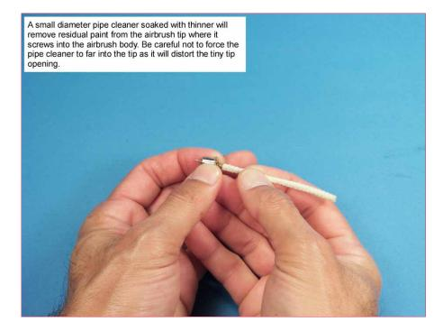
You airbrush should be taken apart after each painting session and the parts soaked in thinner. The individual parts will need to be cleaned, dried and then the airbrush can be reassembled.
