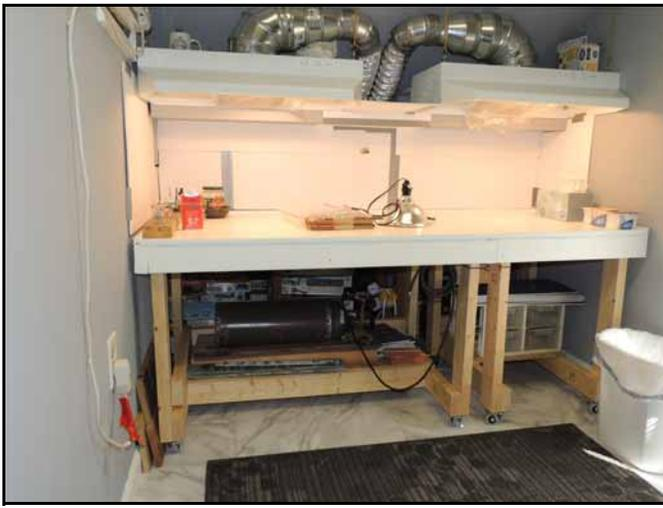
I installed foam board around the work area so that the fumes and paint dust would be more easily sucked out by the ventilators.
