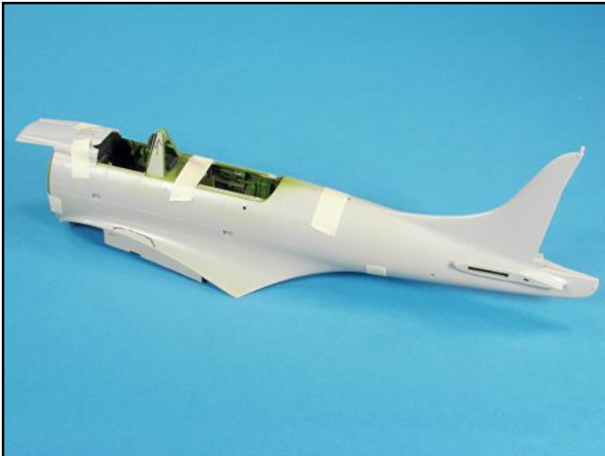
Thanks to all the test fitting prior to assembly and fit checks as the cockpit was assembled, the fuselage halves fit tightly together.
