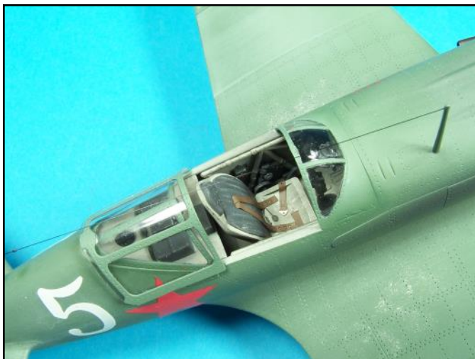
The seat was assembled, the seat belts installed and then the finished seat was carefully glued into place. I used drops of Testors tube glue applied with a toothpick so that I would have some working time to adjust the position of the seat.
