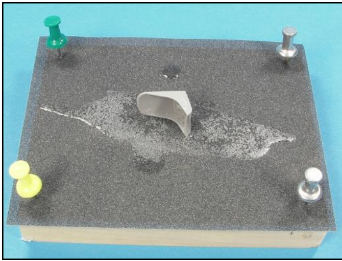
I thinned the sides and the back of the kit supplied seat by running it across a stationary piece of wet sandpaper.
