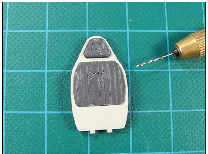
The seat belts come through the seat backing and so to make the rectangular shaped opening, holes were drilled first.
