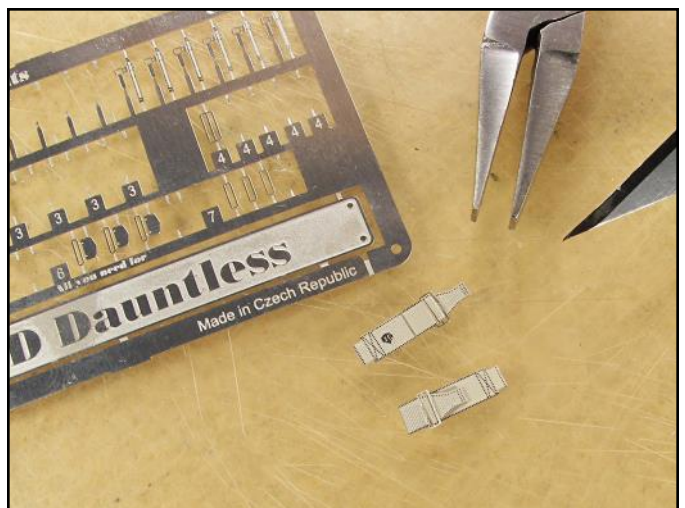
The belts were then carefully bent into shape and the adjusting loops were slipped onto the bent belts and then carefully positioned.
