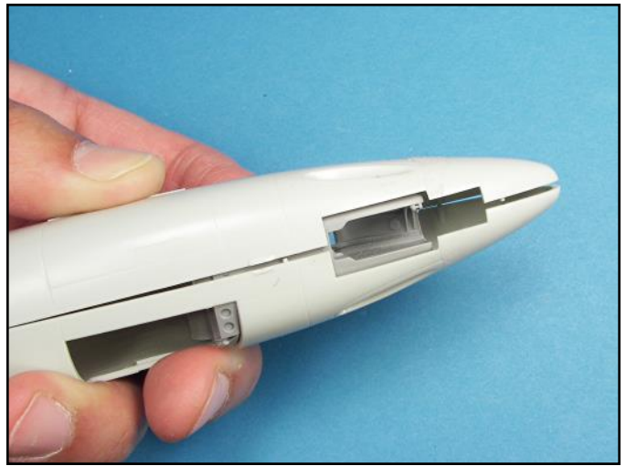
With the resin side walls and cockpit tub taped into place there is a fit problem that will need to be corrected. In this case the cockpit tub was too wide.
