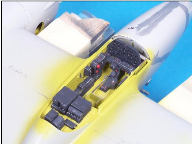
As the cockpit assembly progresses, the console was test fitted and then carefully glued into place with tiny drops of super glue.
