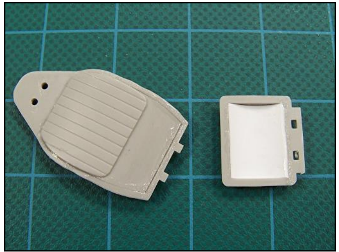
This seat base had some deep mold punch-outs. Rather than trying to fix them, I laminated a piece of .010 inch sheet plastic to the base of the seat. The super glue filled seams on the seat backing were carefully scraped and sanded smooth.
