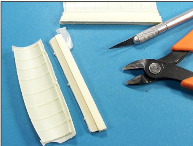
Some types of resin are more fragile than others and snapping the pour plug off might fracture a part. In these cases, cut off the pour plug with a sharp number 11 X-Acto blade.
