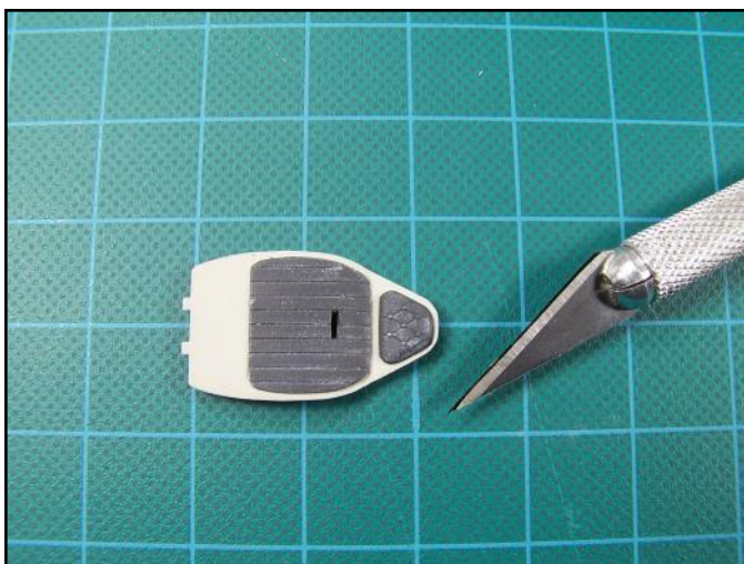
The plastic between the drilled holes were then cut out and micro files were then used to shape and clean the opening.
