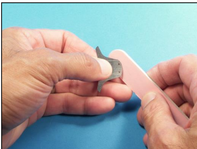
The brass photoetch seat was cleaned up using a sanding stick and then bent into shape and super glued together.
