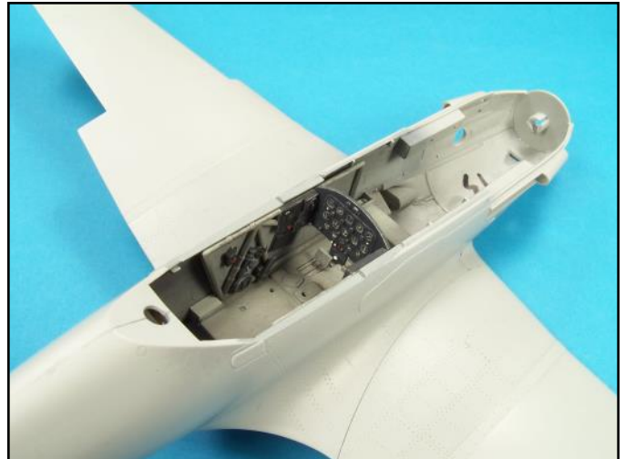
At this point in the construction sequence the fuselage sides were glued together and the instrument panel added. The instrument panel gun sight will be added at a later stage in the fuselage construction sequence.
