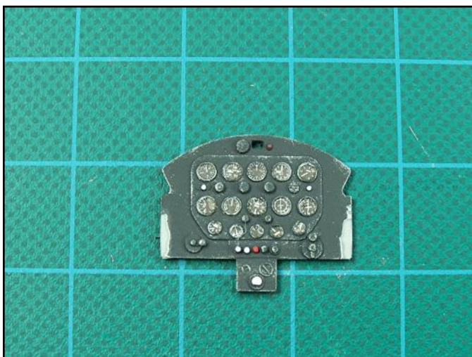
Each instrument also received a drop of white glue so that once dried the instrument appears to have a glass covering. The detail painting was done using a sharp toothpick dipped in the paint cap.
