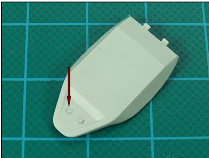
The back of the seat had the positioning pins sticking through. Super glue was applied around the pins and then the pins were cut and wet sanded smooth with fine grit sandpaper wrapped around a length of balsa wood.
