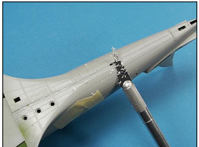
Seam lines along fuselages and wing edges are best scraped first to remove as much of the excess super glue as possible before you wet sand the surfaces smooth. Number 11 X-Acto blades are perfect for this type of work.
