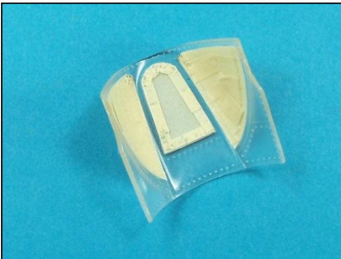
Once the outside area is masked, I mask the inside. I use the outline of the exterior masking tape edges to guide me in the placement of the interior tape.
