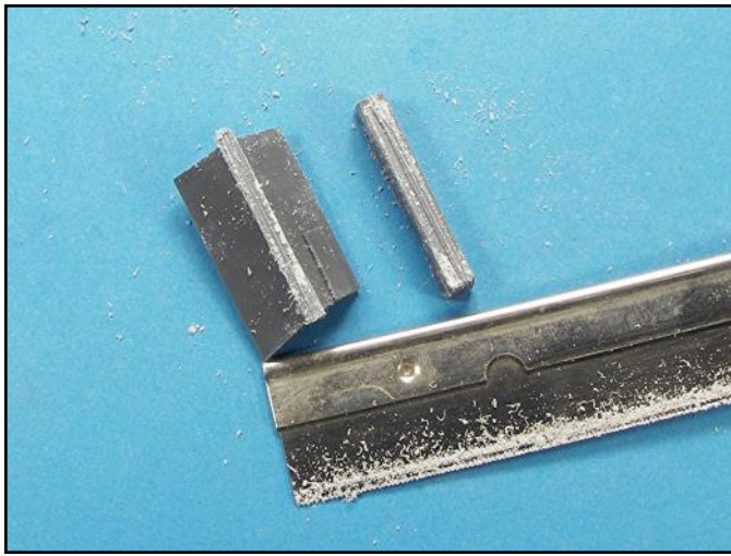
Here is another example of a large resin pour plug that was removed with a razer saw. Always wear a dust mask when cutting resin with a saw, as the dust can irritate your lungs.
