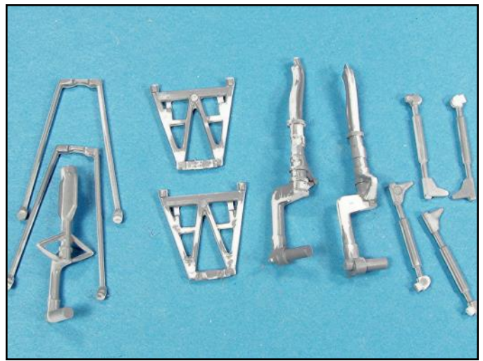
These landing gear parts are white plastic and once primed, a number 11 X-Acto blade was used to scrape the mold punch outs and the mold lines smooth.
