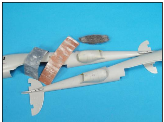
For sanding flat or semi flat surfaces, wrap strips of sandpaper around lengths of balsa wood to smooth out the plastic. Once this is done you can wet sand with finer grades of sandpaper. Polish the plastic with 0000 steel wool.
