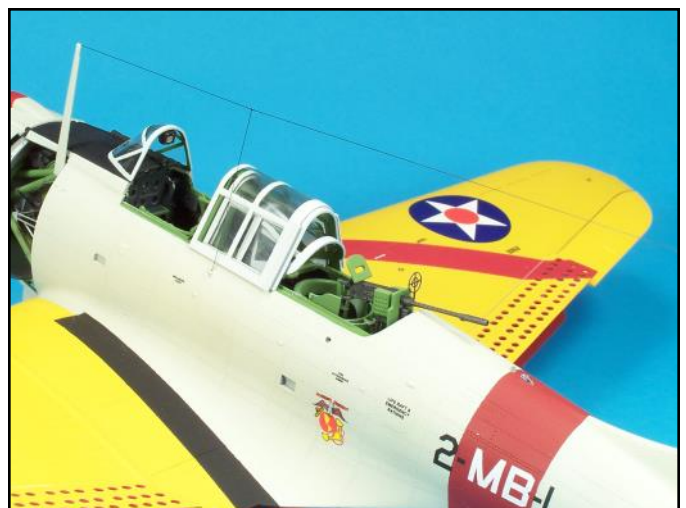
The clear parts on this SBD Dauntless are what I call the "traditional attachment type clear parts." All the canopy parts, including the wind screen are separate and distinct.
