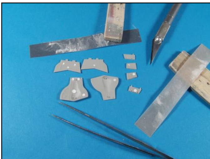
The glued disks were wet sanded smooth with fine grade sandpaper wrapped around lengths of balsa wood. The raised injection marks were carefully scraped with a number 11 X-Acto blade and then sand smooth.
