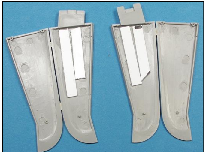
Even small parts can benefit from laminating a few strips of plastic to the inside areas for added strength. Stronger plastic puts less stress on the seams, eliminates cracking and makes the parts easy to handle.
