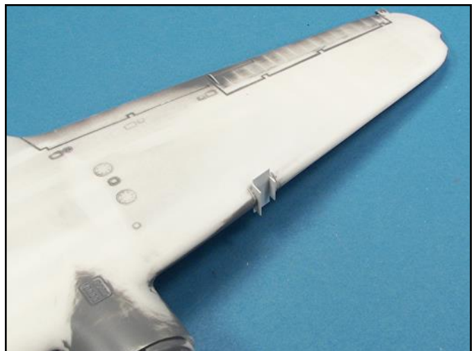
While working with seams, you may have to also address other issues. Sometimes wing lights are openings with a clear plastic cover. Fill the opening with thin strips of plastic attached with super glue.
