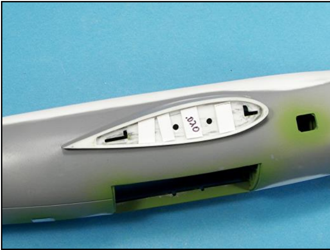
Strips of plastic can also be used to increase a gluing contact surface area and increase the strength of the fuselage to wing connection.
