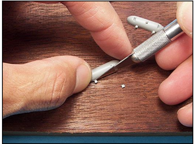
Lay the part flat on a wood block and then cut the remaining stub with a number 11 X-Acto blade.
