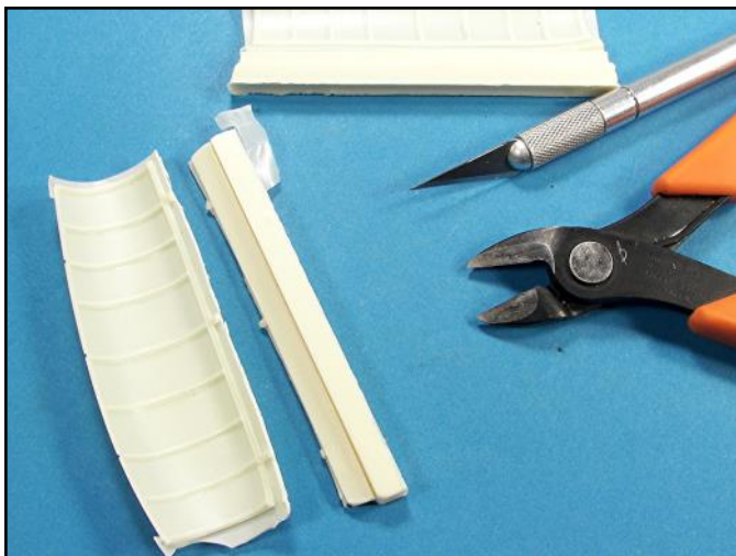
Different resin part shapes require different types of pour plugs. Sometimes you can use a combinations of tools, like cutters and number 11 X-Acto blades to remove the plug and clean up the part.
