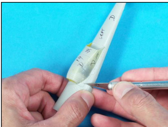
Number 11 X-Acto blades are also great for contouring and scraping parts that do not fit well into their locations. Sometimes you have to remove a lot of plastic to get the parts to fit correctly and make those pesky seams disappear.
