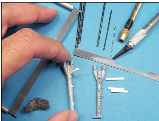
Indented injection marks can be tricky on round surfaces. Drill out the indentation and then super glue round plastic stock into the hole. Trim of the excess and scrape and sand smooth with a Flex-I-File.
