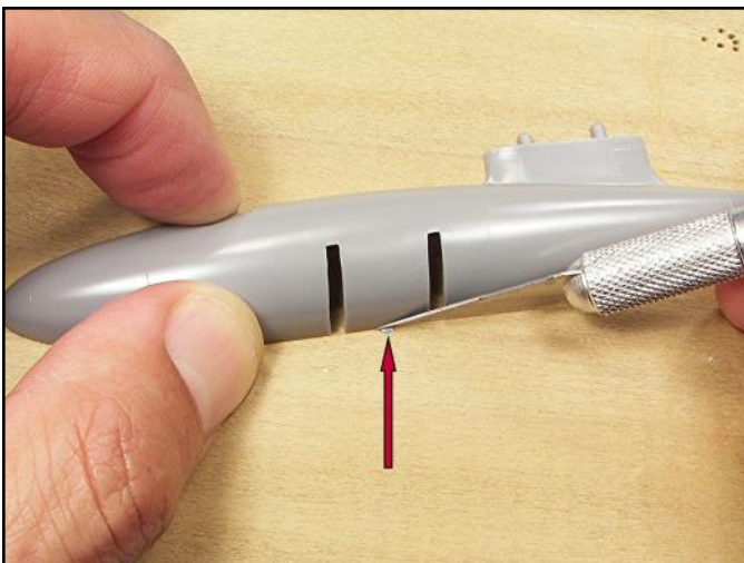
Be careful when cutting a stub off a thin flexible part. Sometimes as you are cutting, the part can flex causing the blade tip to damage the surface of the part.
