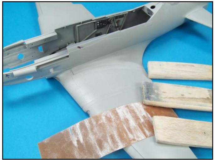
Balsa wood wrapped with sandpaper can also be used to smooth out the seams at wing to fuselage attachment areas. One caution here is that you can easily create a depression if you are not careful, so check your work frequently.
