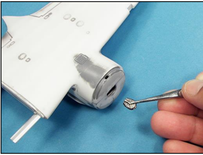
Even the engine nacelles were used to hide small pieces of lead weight to help balance the B-26. To secure the pieces of lead, white glue was squirted into the opening.
