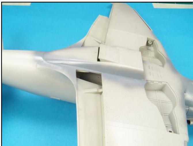
Once the white glue is dry give it a light coat of primer. Check for flaws and repeat the application of the white glue to completely fill the void. Prime the dried glue between applications.
