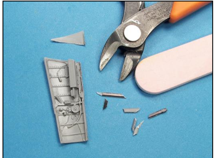
The remaining resin plugs on delicate parts can be removed with snipers and then cleaned up with a sanding stick, if scraping the edge with a number 11 X-Acto blade will damage the part.
