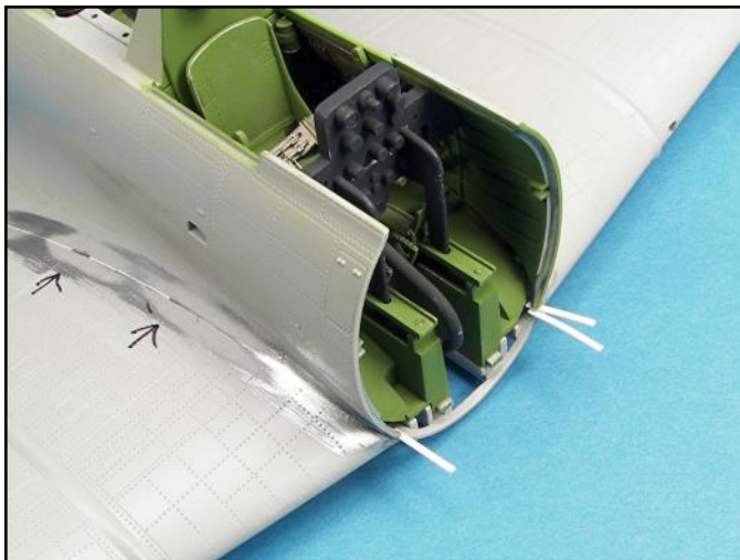
Here is another example of using strips of plastic to fill voids and add strength to the overall assembly.
